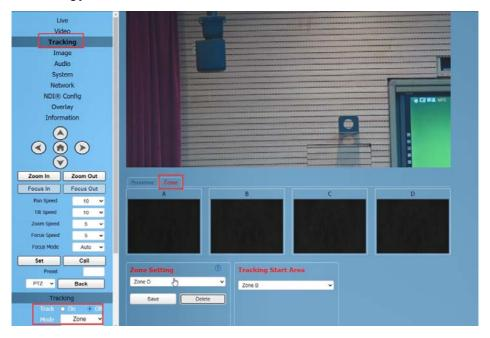
Step 3 Use the web interface's directional keys and Zoom In/Out to adjust the lens position,
