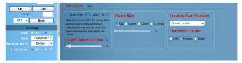
Auto Zoom: Usually remains the default. When "Auto Zoom" is turned off, the camera lens can still move, but can only maintain the current magnification and cannot zoom. Auto Tilt: Usually remains default. When "Auto Tilt" is turned off, the camera lens can only move horizontally.
