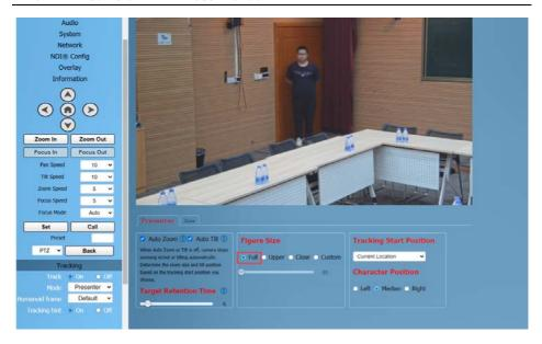
Upper: The close-up image includes tracking the target above the knee, as shown in the following figure.
