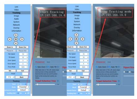
Step 6 Turn on tracking, press the arrow keys to select the tracking target, and then press Home to confirm.
