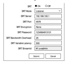
Turn On/Off SRT and set up the SRT Mode, SRT Server, SRT Port, SRT Encryption, SRT Password, SRT Bandwidth Overhead, SRT Variable Latency and SRT StreamID.
